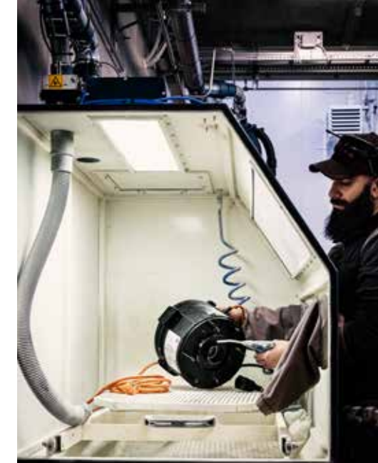
Compressed air connection and blow gun nozzle. Suction hose for easy cleaning inside the cabinet.
